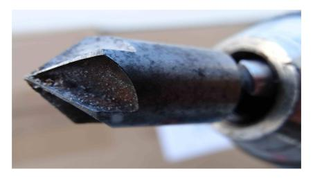
The cabin sides were prepared by countersinking each screw hole. The idea being that the mastic would be compressed into the countersink forcing it around the thread of the screw and, hopefully, ensuring a waterproof seal.
