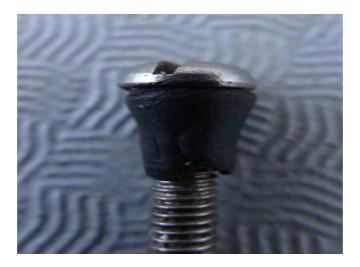
Inside the boat add a washer and nut to each screw and tighten them all finger tight. The windows on FF have a slight curve along the cabin side, it only takes finger pressure to invoke the curve.
